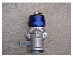
4. Push the plumb back side of the Turbosmart BOV onto the standard return pipe and secure the hose with the provided hose clamp. Unclip the hose shown in the picture from the bracket and move the line under the wiring loom that supports it.
