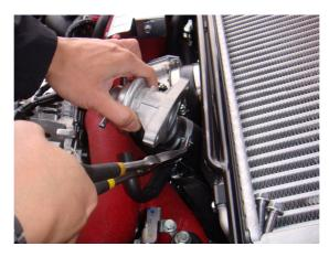
3. Remove the plumb back fitting on the back of the standard BOV and install it onto the Turbosmart BOV using the standard screws.
